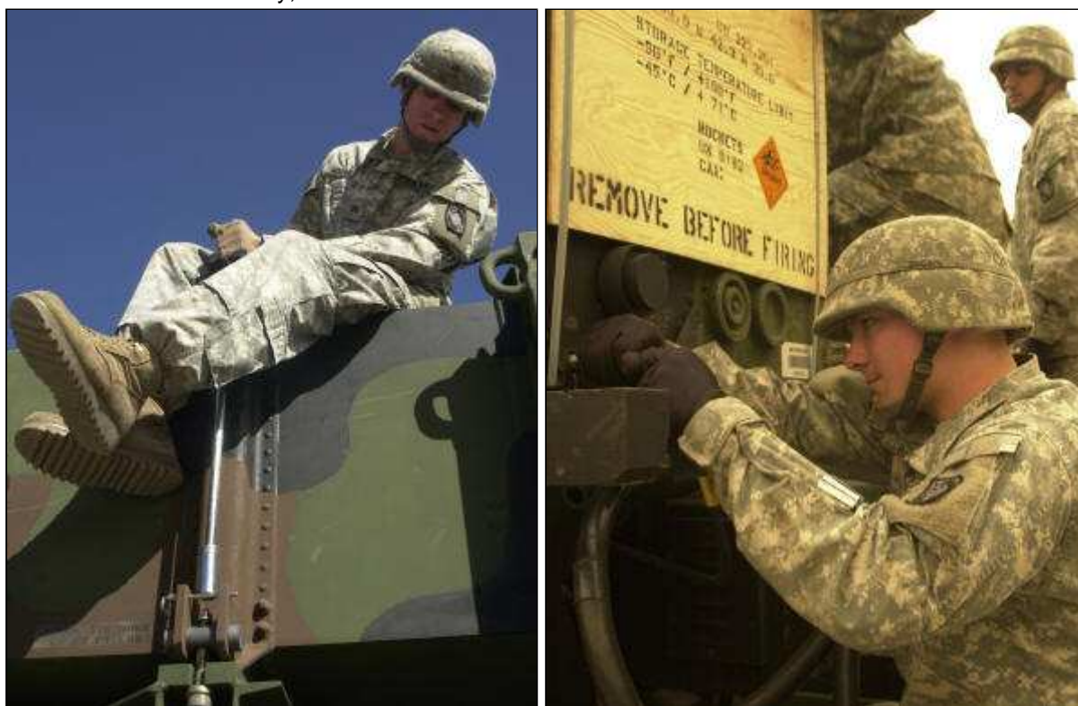
At left, Pfc. Robert Brown of Bravo Battery, 5th Battalion, 7th Air Defense Artillery, attaches a grounding wire to a Patriot missile canister after it has been loaded on to an ammunition truck at the NATO Missile Firing Installation on the Greek island of Crete. With the final turn of a torque wrench, Pfc. Michael Hibdon, right, of Delta Battery, 5th Battalion, 7th Air Defense Artillery makes sure the missile canister safely secured to the launching station. (U.S. Army photos by Staff Sgt. John Queen, 69th ADA Brigade Public Affairs)
